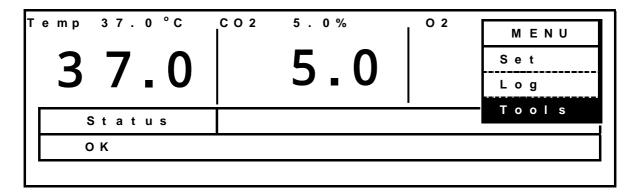
**2.** Select *Temp/CO2/O2 Calibration* from the Select Tools Display, press the MENU Key to display the menu, select *OK*, and press the ENTER Key.
